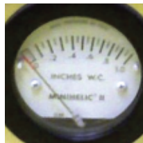
SPM Static Pressure Monitor (3" Dia. Gage)
